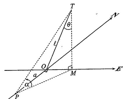
A pole,  $OT$ , of length  $\ell$  m, stands on horizontal ground. The pole leans towards the east, making an angle of  $\theta$  with the vertical. From  $P$ ,  $a$  m south of  $O$  the elevation of  $T$  is  $\alpha$ .
